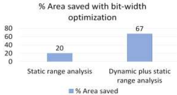
Figure 4: Percentage area saved on FPGA with static and dynamic range analysis for bit-width optimization
