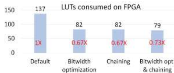
Figure 5: LUT consumption on FPGA for default HLS configuration, with bit-width optimization (static and dynamic range analysis) enabled, with chaining enabled and a combination of bit-width optimization and chaining enabled, in this order from left to right.
